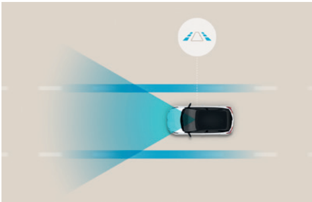
Lane Following Assist (LFA). When activated, it keeps the vehicle centred in its lane at speeds between 0 and 200 kilometres per hour on highways and city streets.
