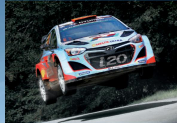
The hand-built i20 WRC is a high-performance competition car based on the popular production vehicle. Developing more than 300 PS of power and 400 Nm of torque from a 1.6-litre engine and weighing 1,200 kgs, it requires highly-skilled drivers and co-drivers to handle its immense power
