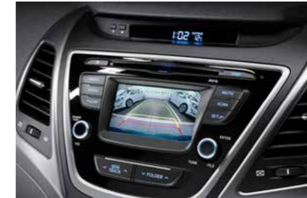
Reverse Camera. When reverse gear is selected the camera feeds a live view of the area behind the car to the 4.3" TFT LCD audio display.
